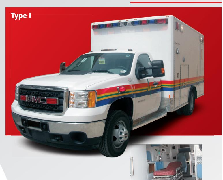
This is a modular ambulance built on a truck chassis. A key advantage to the Type I is that the module can be remounted on a new chassis when the initial chassis is worn out. It is a cab and chassis customized modular ambulance that is designed to provide more space inside, while having exterior compartments for storage of generators, oxygen cylinders and other specialty equipment.
