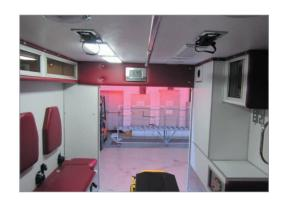
This is a modular ambulance built on a truck chassis. Type III features a walkthrough bulkhead, allowing for passage between patient compartment and cab. The conversion can be remounted and be installed with similar medical equipment.
