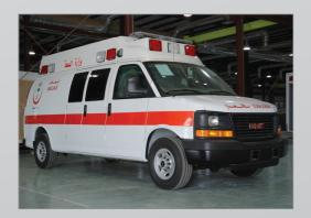
This is an urban response ambulance using a van-type chassis. The remarkable modifications of the van are the addition of a metal rollover safety cage and reinforcement of the interior walls, and then interior headroom is raised by adding cold formed rollover-cage system that is topped with insulated fiberglass. This type can be equipped either with efficient Advance Life Support (ALS) or Basic Life Support medical equipment.
